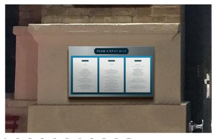
10MM THICK EXISTING PLUM & SPILT MILK SIGN RELOCATED TO THIS POSITION AND TO BE FLUSH MOUNTED ONTO WALL WITH VHB TAPE. NON-ILLUMINATED
