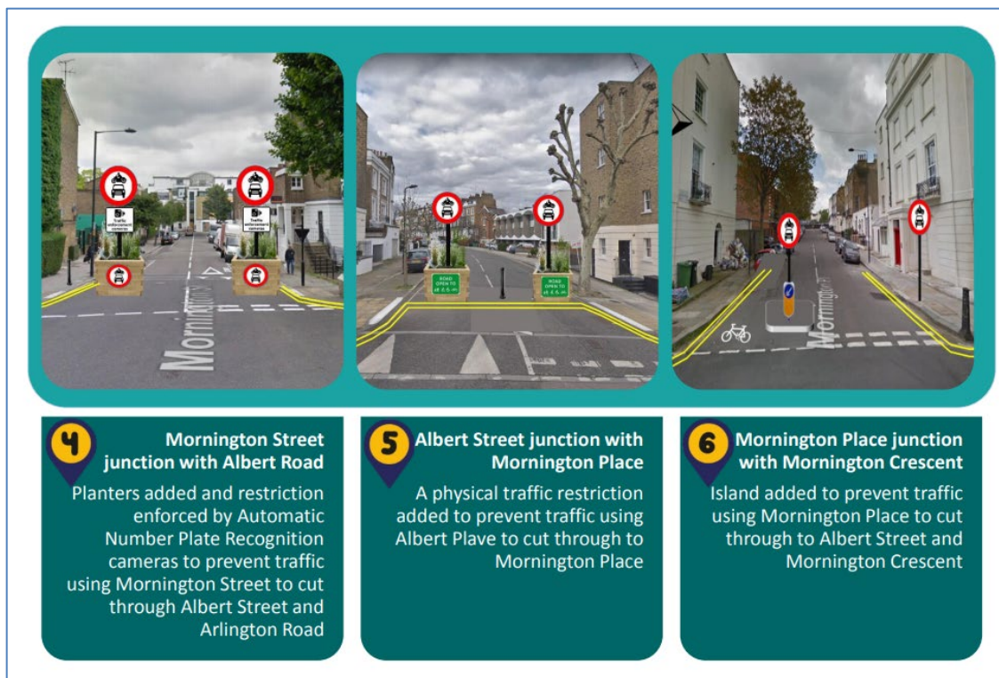
Figure 2.3: Planned Safety Improvements to Arlington Road Area
