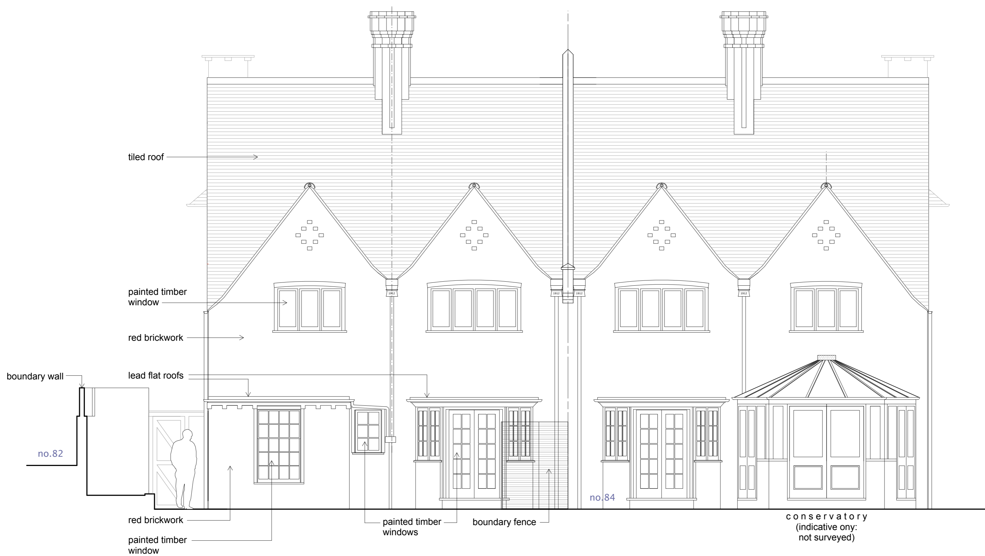
REAR ELEVATION AS EXISTING
