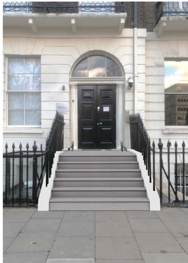
Fig.2 Proposed over- clad yorkstone steps
