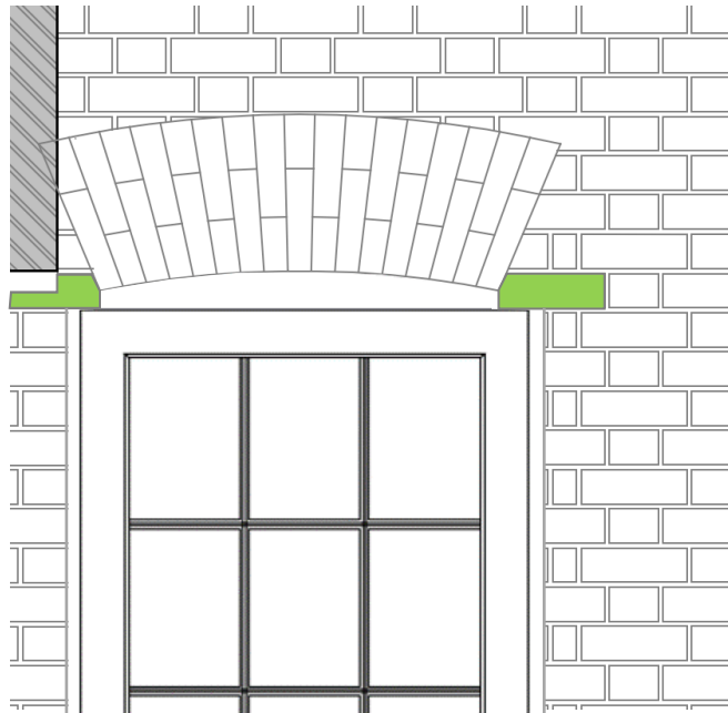
OPTION 2 : USING A PROPPED ARCH METHOD
