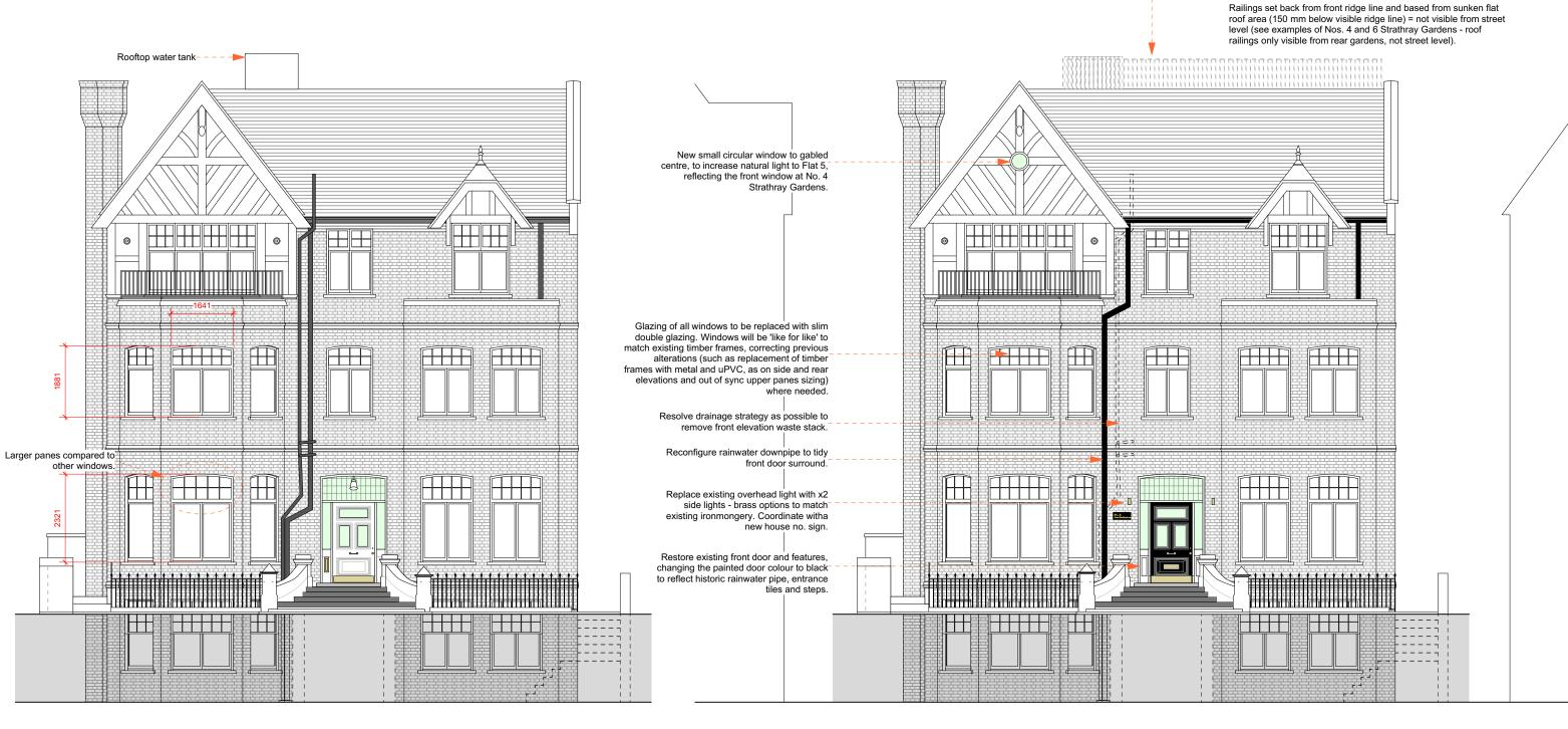
Roof access safety railing and water tank hoarding - black metal railings to match existign railings elsewhere at the property.
