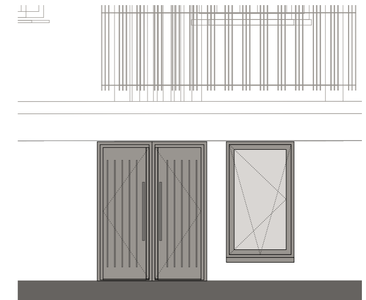
Typical Riser cupboard access doors in Underbuilds
