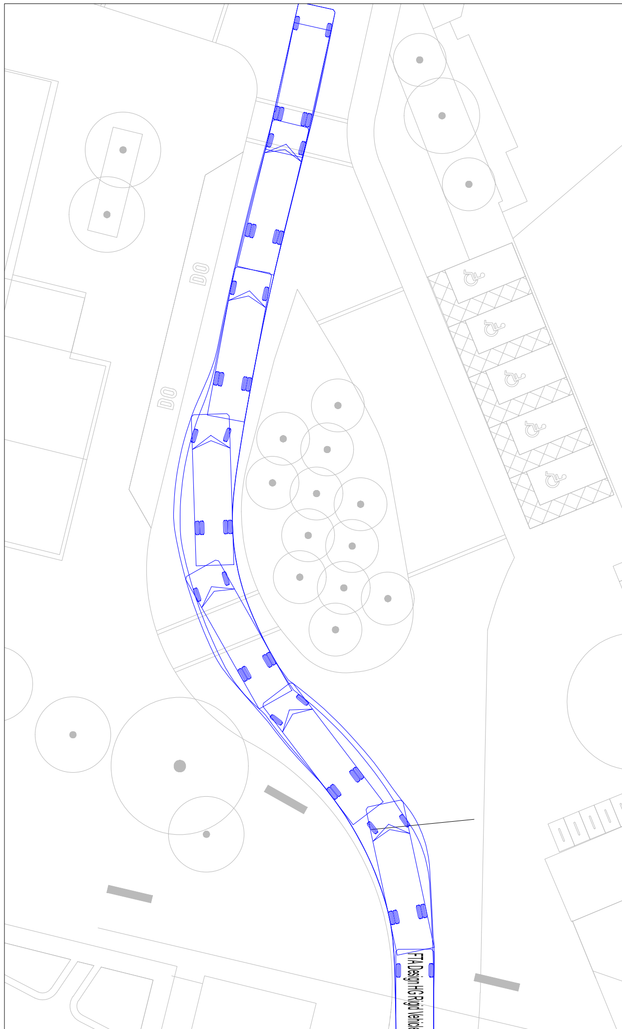
7.5t BOX VAN EXITING BASEMENT
