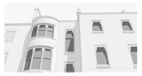
Figure 38: Visualisation of proposed raised bay parapet
