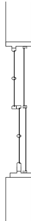
Typical Section through vertical sash windows
