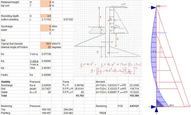
Permanent case head of wall restrained by ground floor slab Moment per piles = 38.5kNm
