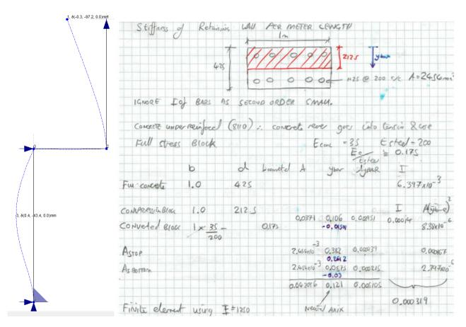
Analysis model based on Stiffness of 1250 in steel, the above is a cracked I value for the concrete section Deflection  $97.2 \times 1.250x-5 / 0.00039 = 3.75$
