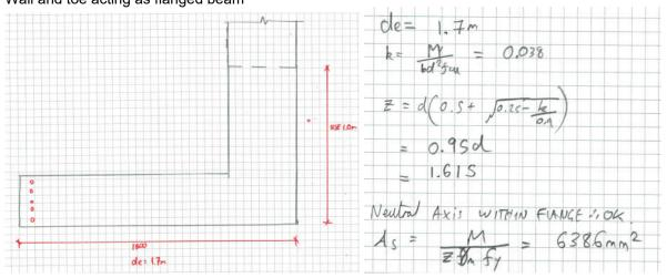
Use 10 H32 bars = 8042 mm<sup>2</sup> within pile cap to form horizontal beam to provide restraint to wall and pile cap/ Retaining wall to have H16 bars at 200 centres
