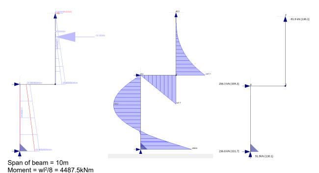
Wall and toe acting as flanged beam
