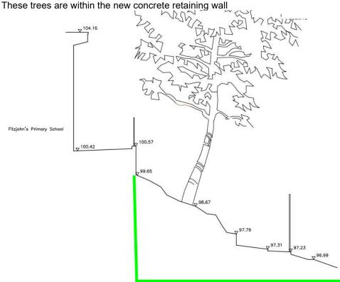
The new building will be founded on a piled raft and therefore designed to be resistant to the effects of these tree removals.
