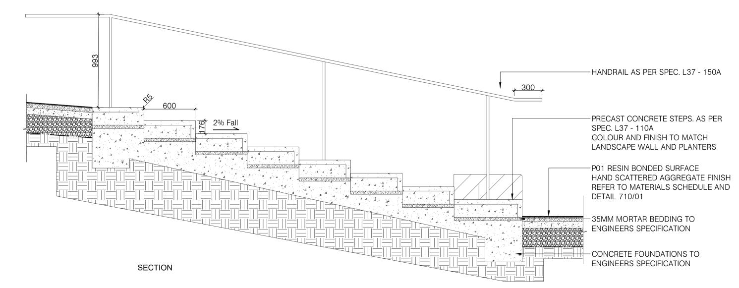
TYPICAL SECTION THROUGH RETAINING WALL STAIRCASE SCALE :1:20 @ A1
