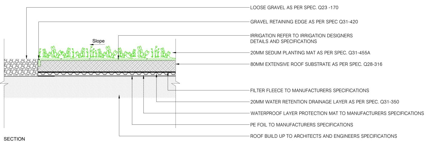
O1 TYPICAL GREEN ROOF SECTION AND PLAN
