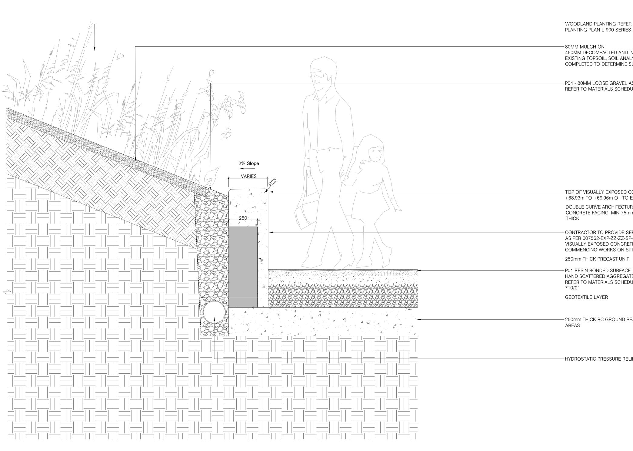
01 TYPICAL SECTION THROUGH RETAIING WALL SCALE :1:10 @ A1
