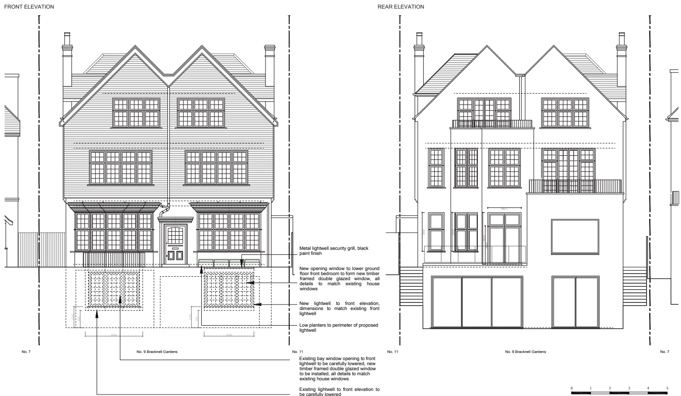
Front and rear elevation drawings showing the existing left hand and proposed right hand lightwells, and the existing 2 storey extension to the rear.
