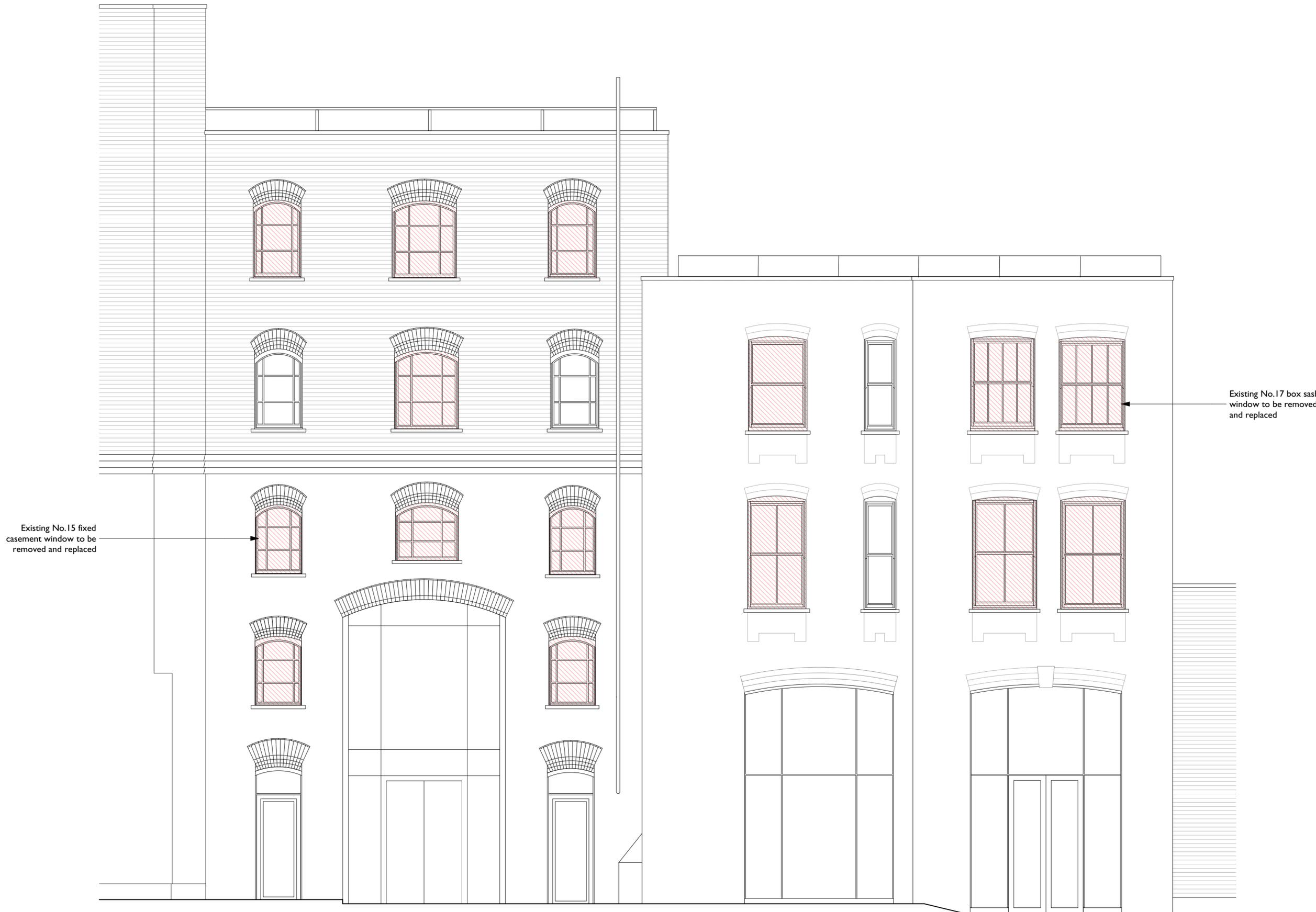
Existing No. 17 box sash window to be removed and replaced
