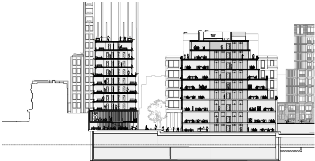
Figure 4 - Extract from the planning application elevation and section drawings showing the proposed hotel and double basement underneath (note the Ear Institute is not shown on this section)
