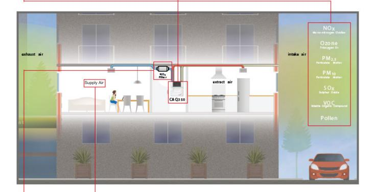
The NO<sub>x</sub> high grade filters are placed within the supply air network. Air enters the dwelling and is filtered via the Heat Recovery System (G4) and then through the high grade carbon filter to remove the hazardous particles.
