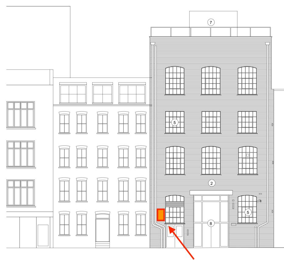
Facade, bracket mounted AQ monitor unit, min. 0.5m from face of facade, min. 1.5m above ground level
