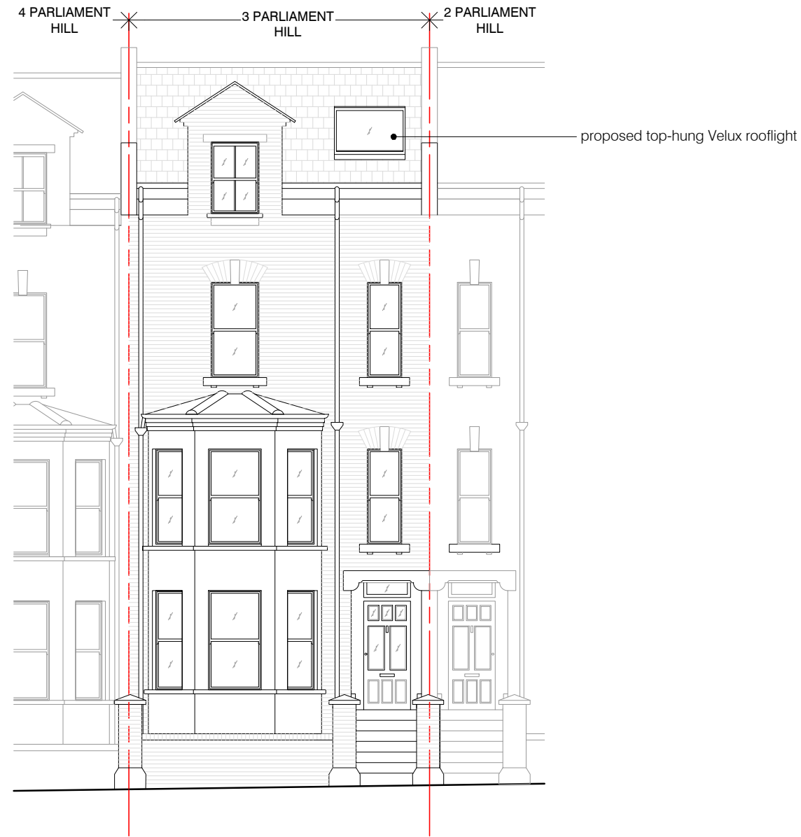
01 PROPOSED FRONT ELEVATION scale 1:100
