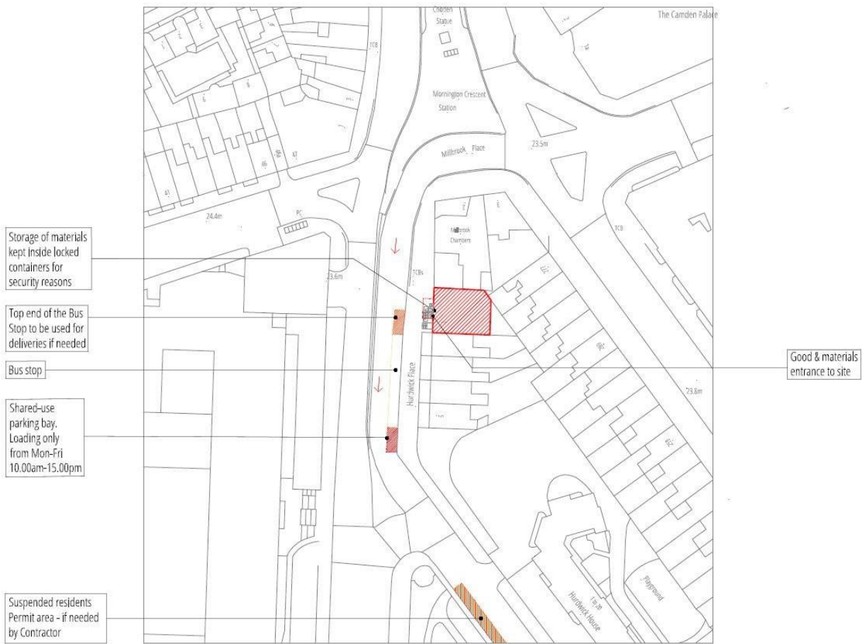
Fig 1 - Parking Plan showing shared use parking bay outside no. 5 Hurdwick Place and additional options if required by Contractor.
