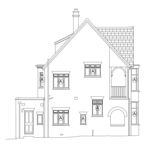
All existing (timber/aluminium, steel and UPVC) windows to be replaced in painted timber double glazed casement windows to match proportions and profile of existing windows.
