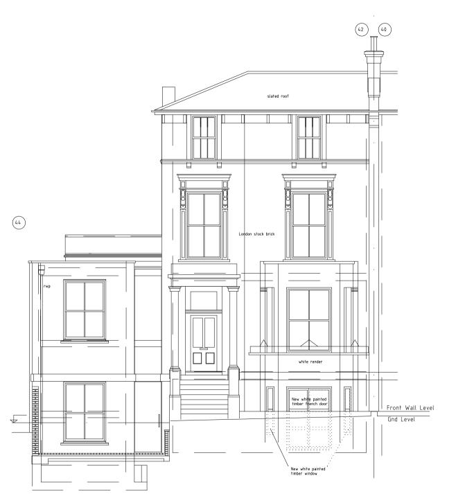
Bay Window Replacement with French Doors and Reglazing of Previously In-Filled Side Bays
