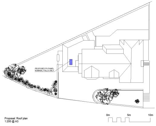
The panel is located in a flat position on part of the flat roof which will have no visibility from the public realm. Photovoltaic/Solar panels are a low-carbon energy source and will be sized to secure a approximately 20% of the energy supply for the new building.
