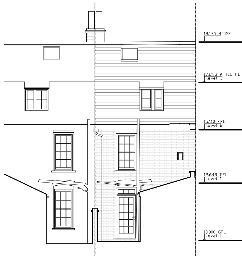
EXISTING Rear Elevation 2-2 1:100@A3
