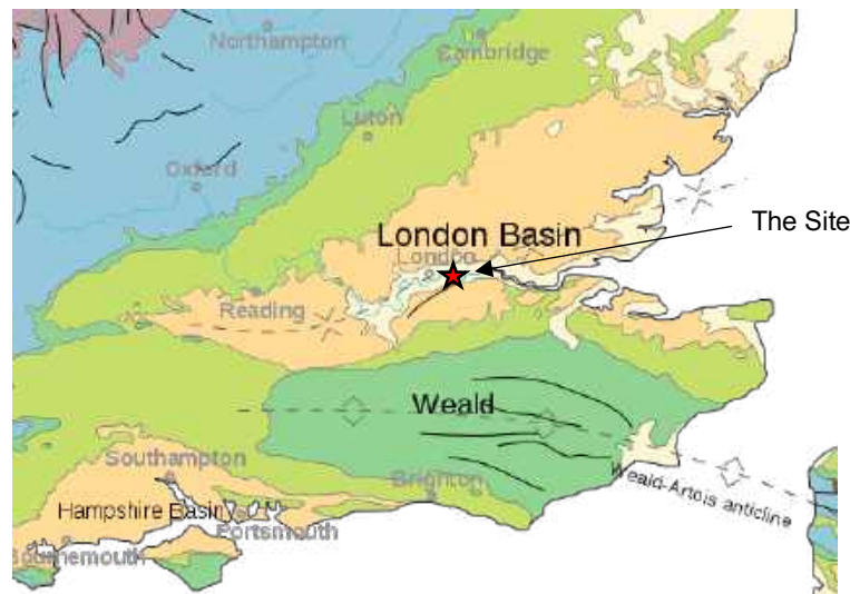
Figure 3.1 Relationship between the synclinal London Basin and Wealden anticline
