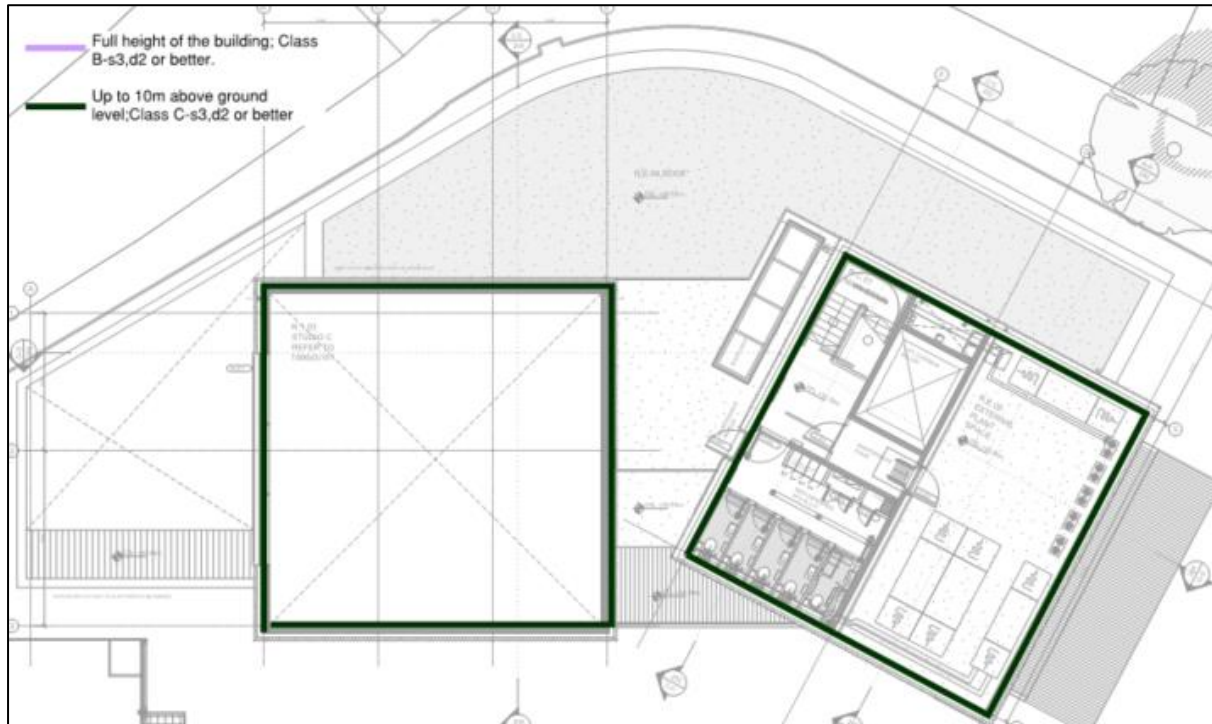
Figure 6 - External wall surfaces- reaction to fire performance requirements (Second floor)
