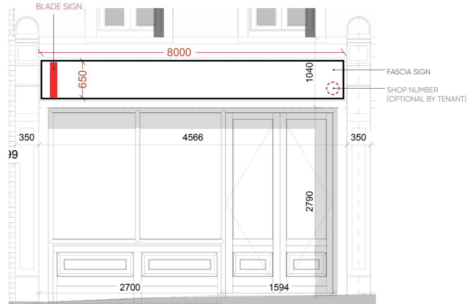
TYPICAL BAY ELEVATION *ALL DIMENSIONS ARE IN MILLIMETRES
