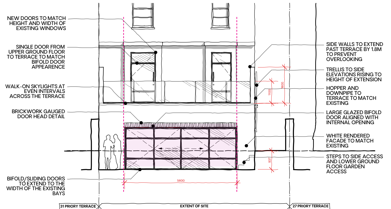
Fig.36 Proposed extension framing to existing rear bays and internal openings
