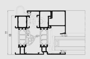
Concept System® 77 is a high insulation window and door system that meets elevated requirements regarding thermal insulation, stability and security. The system's HI+ variant achieves Uf values down to 1.2 W/m²K. The Uf value of a frame/vent section with 115 mm visible width is 1.7 W/m²K.
