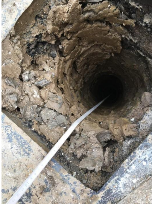
Plate 6 – TAPE MEASURE CONFIRMING BOREHOLE DEPTH AT 10M
