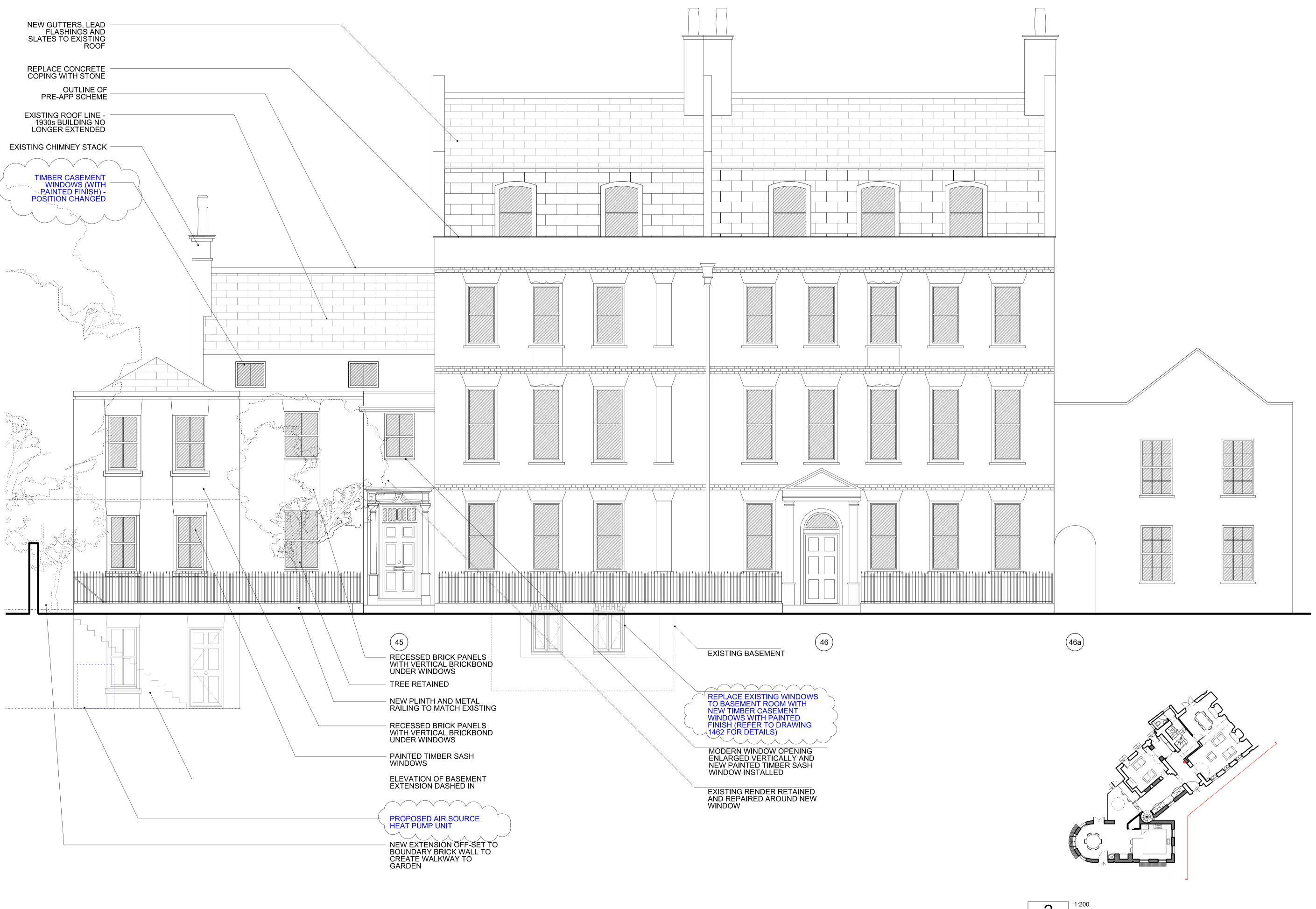
PROPOSED FRONT ELEVATION (FLATTENED) STATUS PLANNING CHECK
