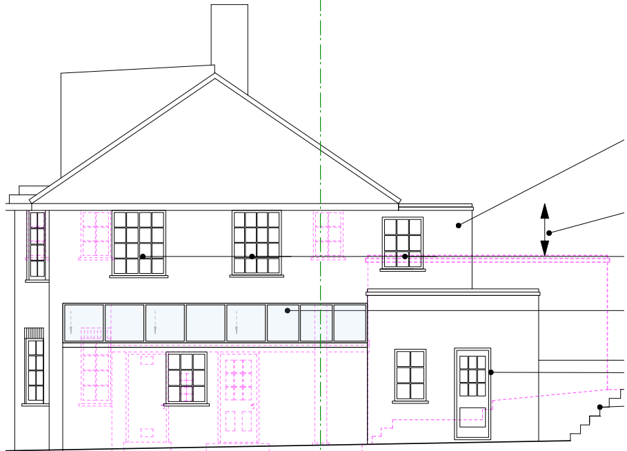
(side elevation, showing replacement side extension)
