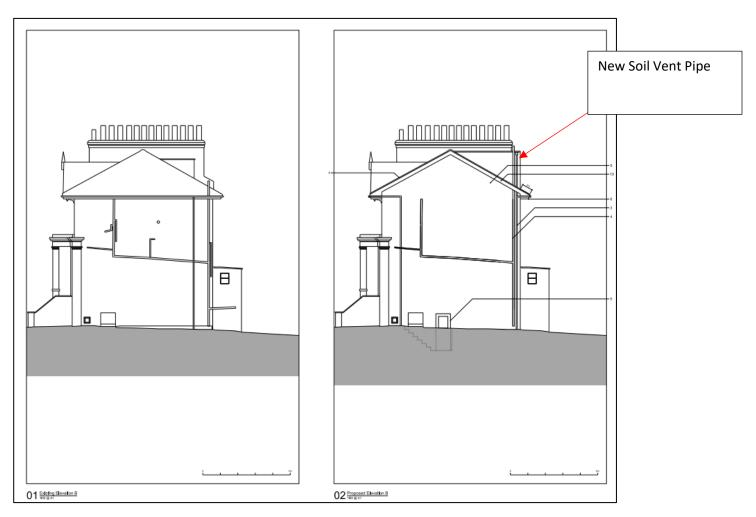
As shown on the proposed drawings, a soil vent pipe would be installed on the side elevation of the dwellinghouse contrary to B. 1 (e) of the Town and Country Planning (General Permitted Development) (England) Order 2015 (as amended).
