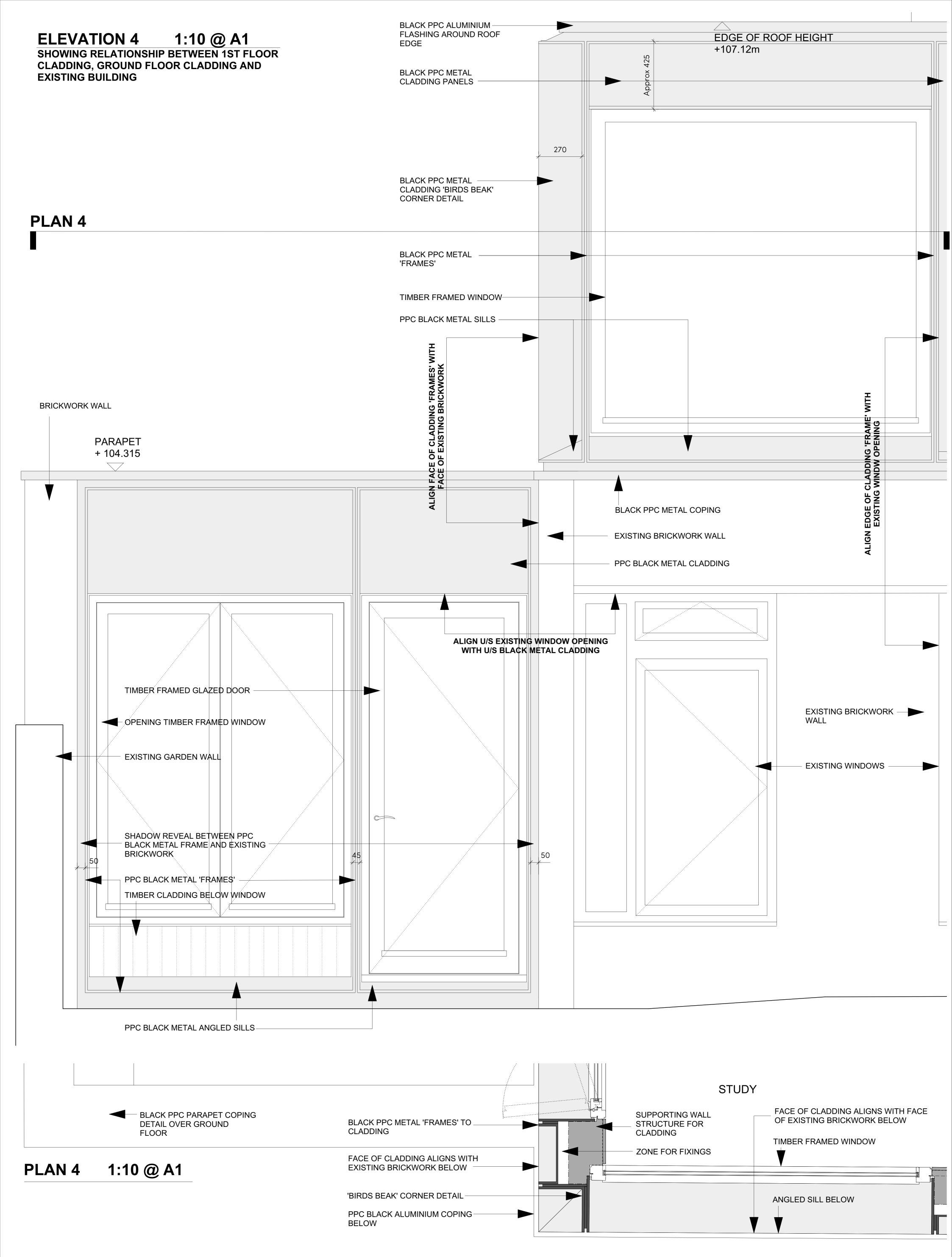
SOUTH EAST ELEVATION AND PLAN SHOWING CLADDING RELTIONSHIP WITH EXISTING BUILDING 1:10 @ A1 5A TEMPLEWOOD AVENUE 25/05/21
