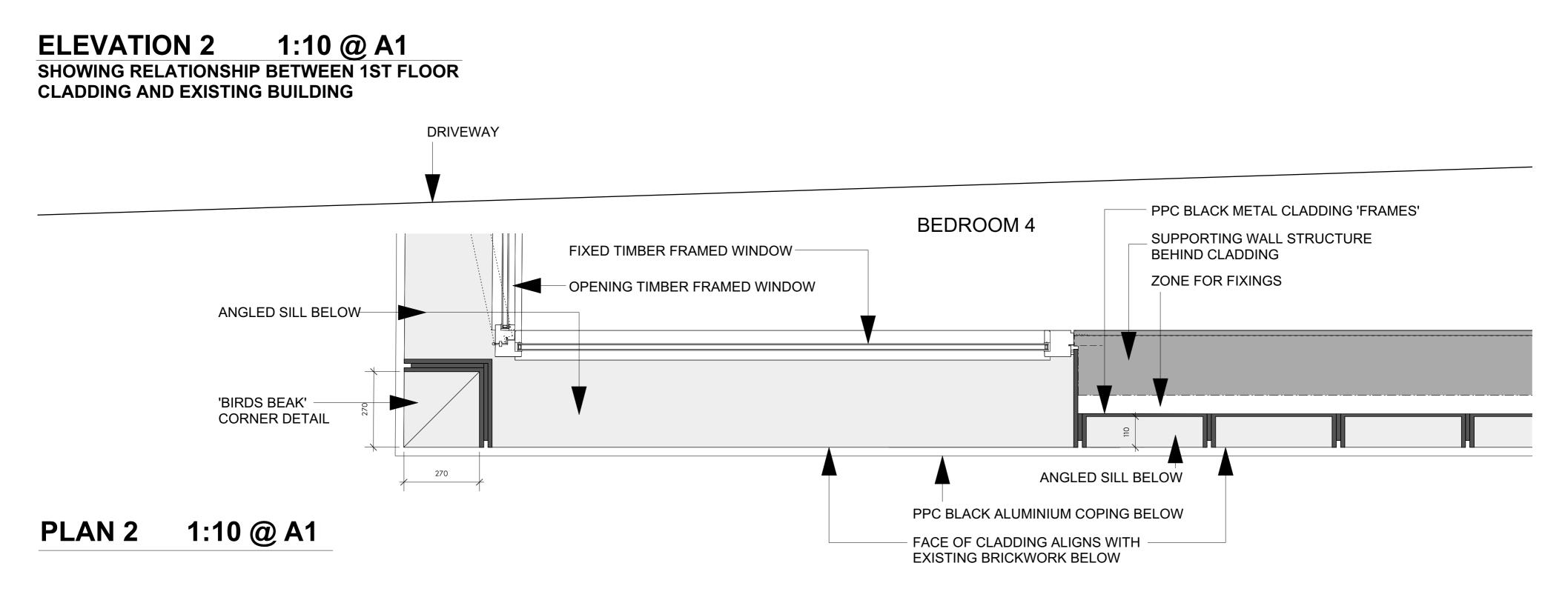
NORTH EAST ELEVATION AND PLAN SHOWING CLADDING RELTIONSHIP WITH EXISTING BUILDING 1:10 @ A1 5A TEMPLEWOOD AVENUE 25/05/21
