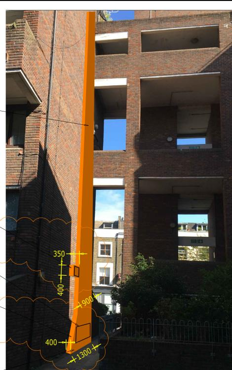
3RD FLOOR BRANCH PIPEWORK.— SEE DRAWING i1237/M/DET/SF5/3
