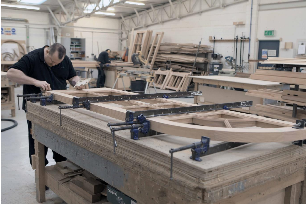
One of our traditionally skilled bench joiner's forming a window casement
