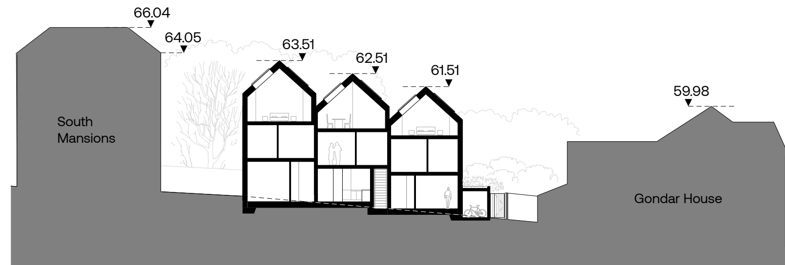
DIAGRAM - SECTION Roofs and floor plates stepping down
