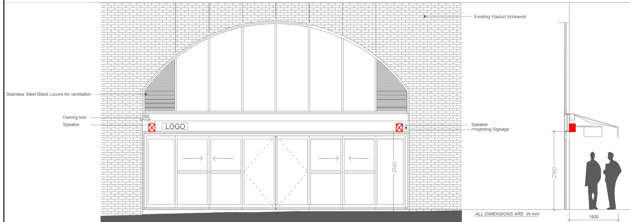
TYPICAL F&B UNIT FRONT ELEVATION (S 15 arch with 2 fascia mounted speakers) (Shopfront strategy under condition 21 of planning permission 2012/4628/P , approved on 13 February 2020)
