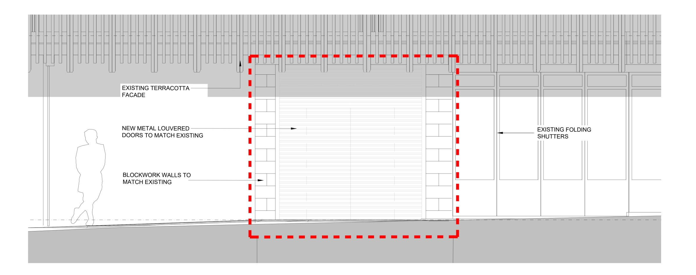
DOOR ELEVATION - A2 PROPOSED SUBSTATION SCALE 1:25 @ A1
