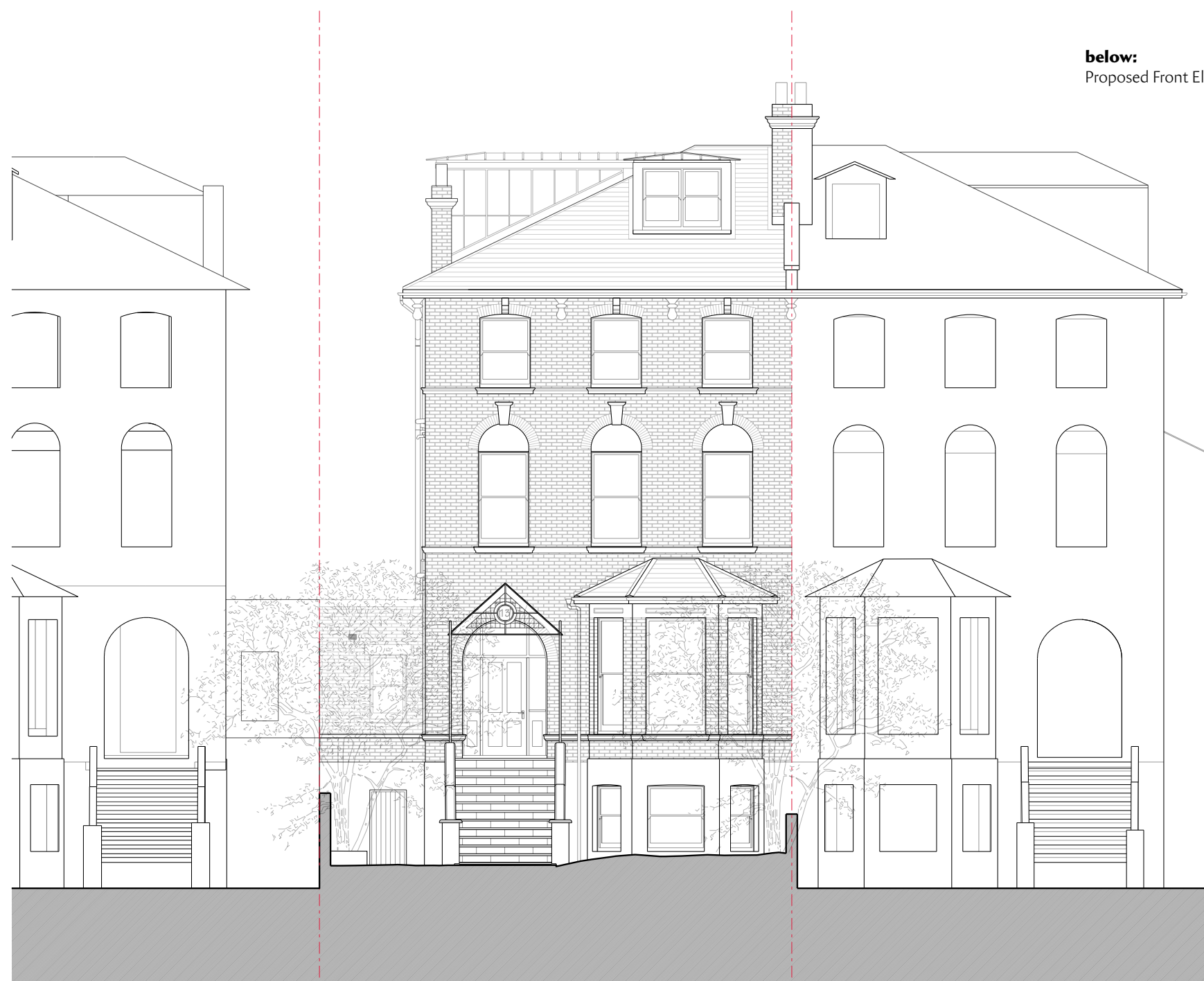
diagram 1: Schematic view of elevation along south side of Elsworthy Road showing prevailing precedent of infill extensions.
