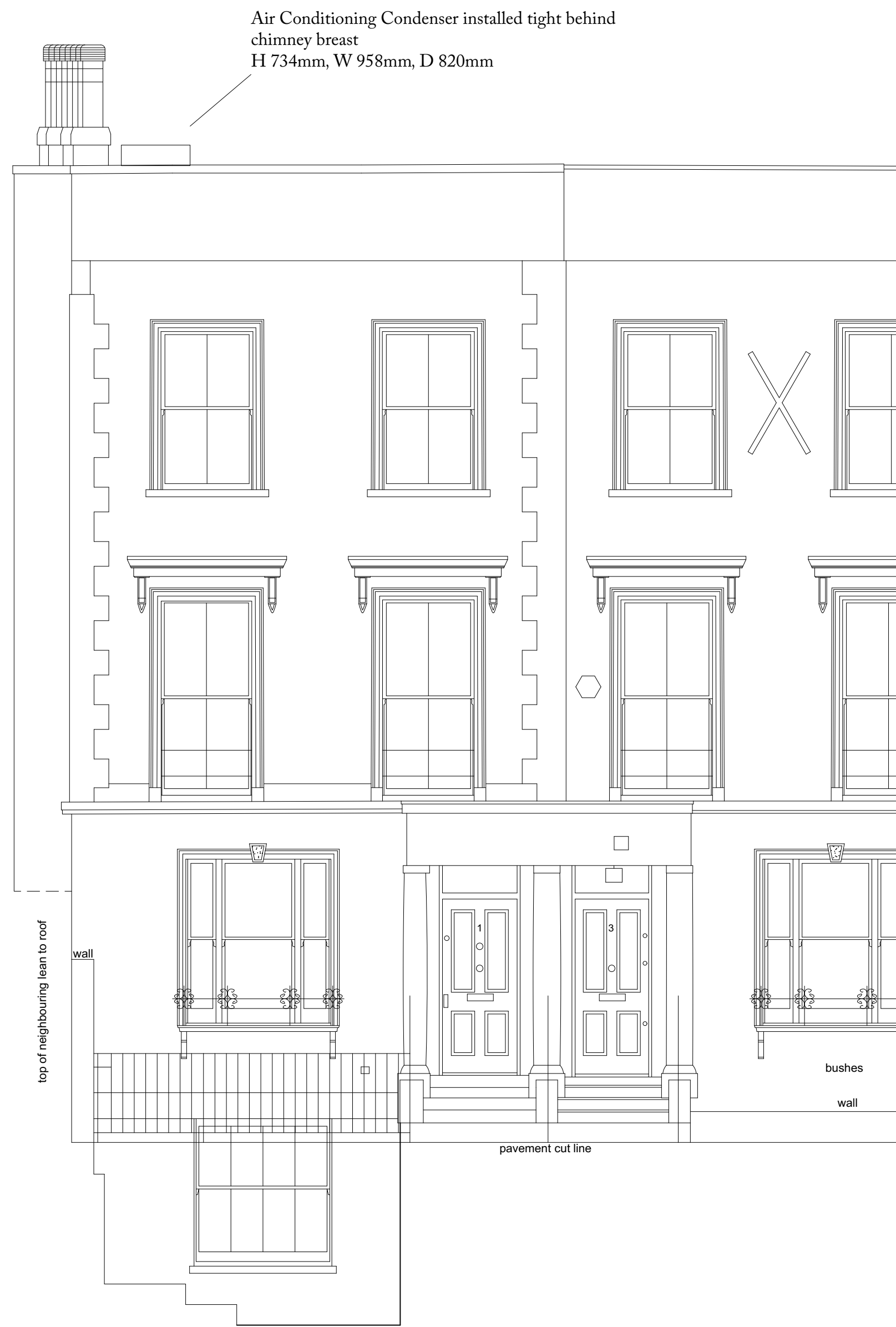
1 EXISTING FRONT ELEVATION 1:100 @ A3
