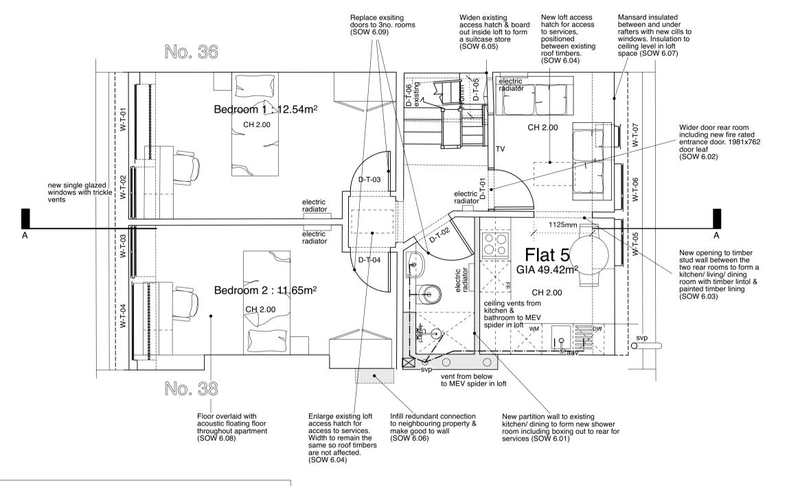
KEY Proposed new partitions & walls with new doors Service walls to rear of kitchens - not full height CH X.XX Proposed ceiling height Foul drainage runs Door - floor - number D-XX-XX W-XX-XX Window - floor - number Cross reference to Schedule of (SOW X.XX) Works in Heritage Statement
