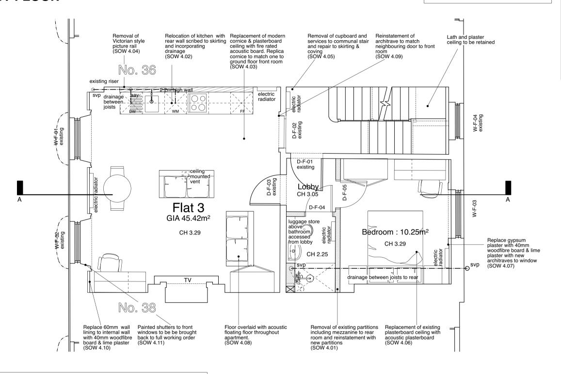
Proposed new partitions & walls with new doors Service walls to rear of kitchens - not full height CH X.XX Proposed ceiling height Foul drainage runs Door - floor - number D-XX-XX W-XX-XX Window - floor - number Cross reference to Schedule of (SOW X.XX) Works in Heritage Statement
