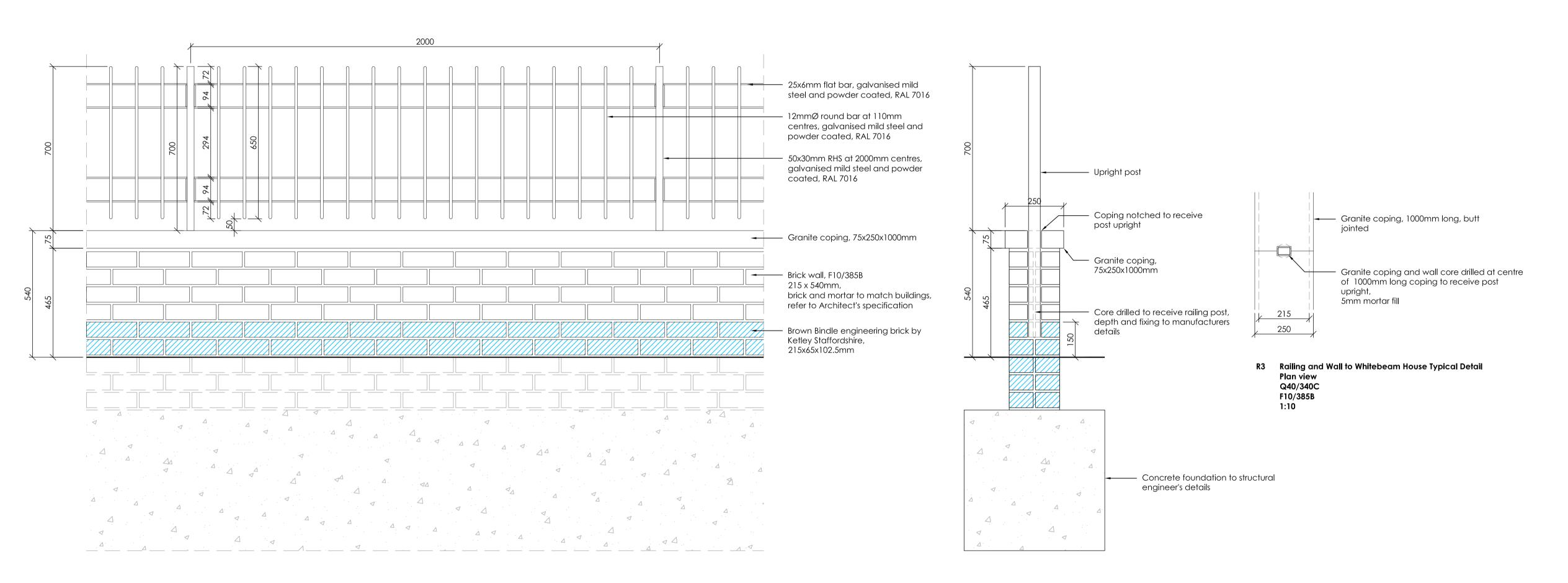
R3 Railing and Wall to Whitebeam House Typical Detail Elevation Q40/340C F10/385B 1:10
