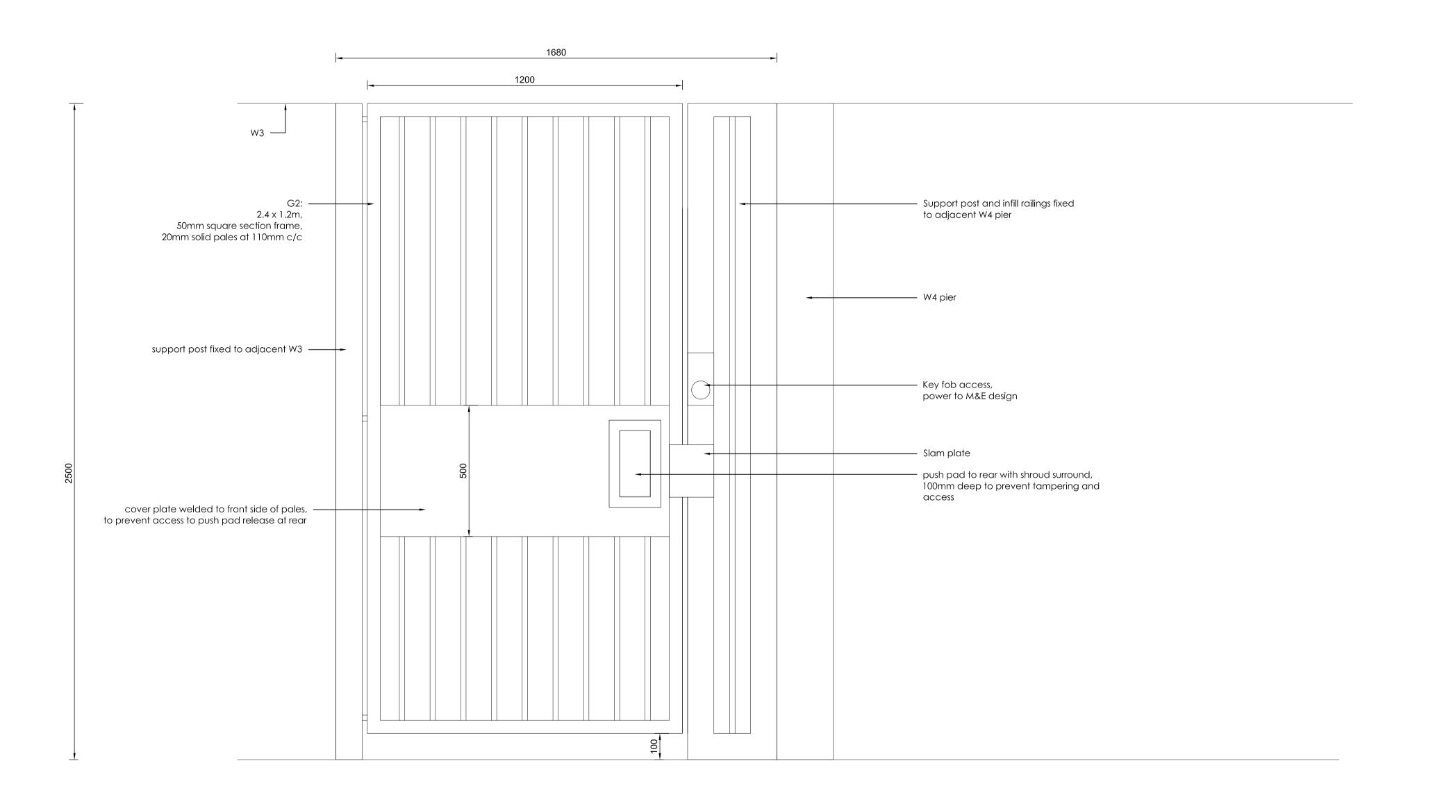
G2 Steel Gate Typical Detail Elevation from inside Q40/570B 1:10
