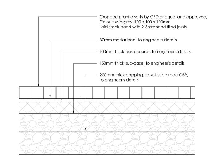
P9 Cropped Granite Paving Build-up Detail Q25/330A 1:10
