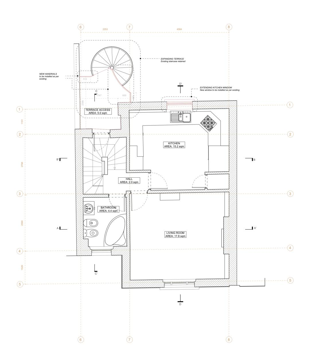
01 PROPOSED FIRST FLOOR PLAN 1:50 @ A1, 1:100 @ A3
