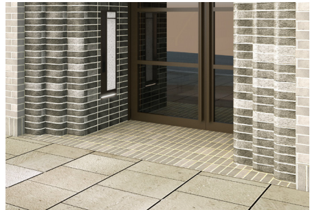
3 Brick continues as floor finish at external threshold
